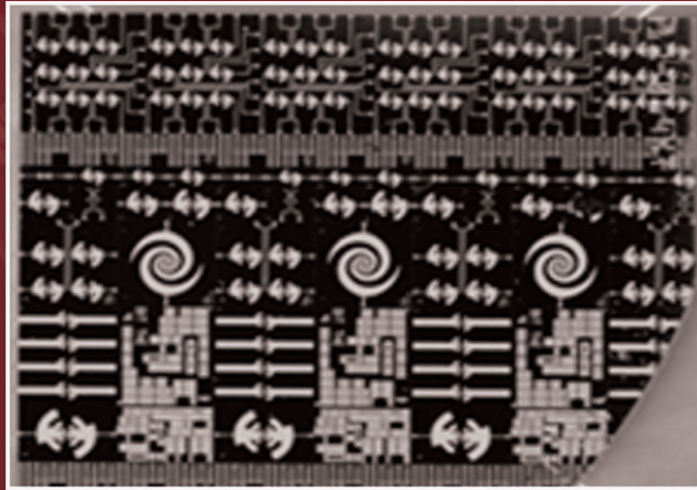
Terahertz technology: monolithic integrated circuit of Schottky diodes and quasi-optical mixer/detector
